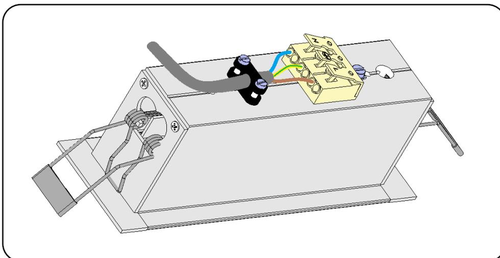
**STEP 3 :** Push both spring clips backwards. Now press the parts with the flat plates inwards and feed them into the opening in. The short parts remain outside the opening. Now push the fixture inward.
