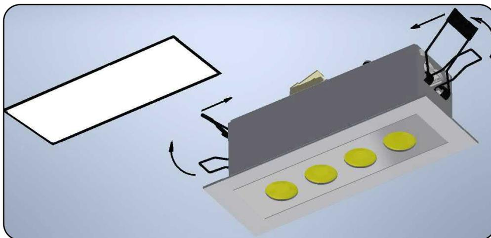
**STEP 4 :** The spring clip (a) will end up with the short part on the side of the opening and the large part with the flat plate will clamp the fixture against the construction plate (b)
